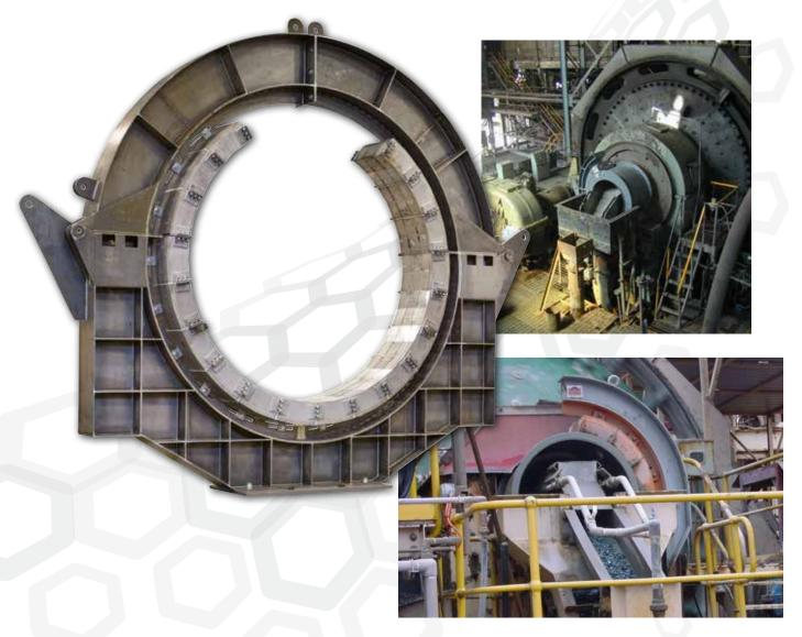
PERMANENT MAGNETIC SEPARATION SYSTEM FOR THE AUTOMATIC AND CONTINUOUS REMOVAL OF GRINDING BALL CHIPS/SCATS FROM THE SAG/BALL MILL DISCHARGE
